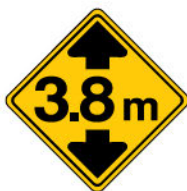
Underpass ahead Overhead clearance as shown
