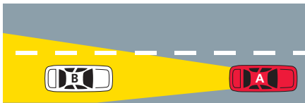
Using the inside rear view mirror, the driver of vehicle A can see vehicle B.
