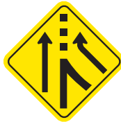
Free flow (added lane)
